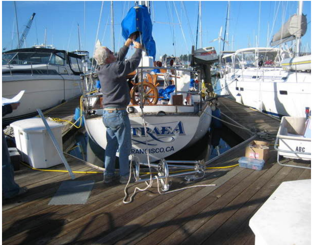
Tim prepares a hoisting line from the mizzen boom to raise the heavy Monitor Wind Vane frame.
